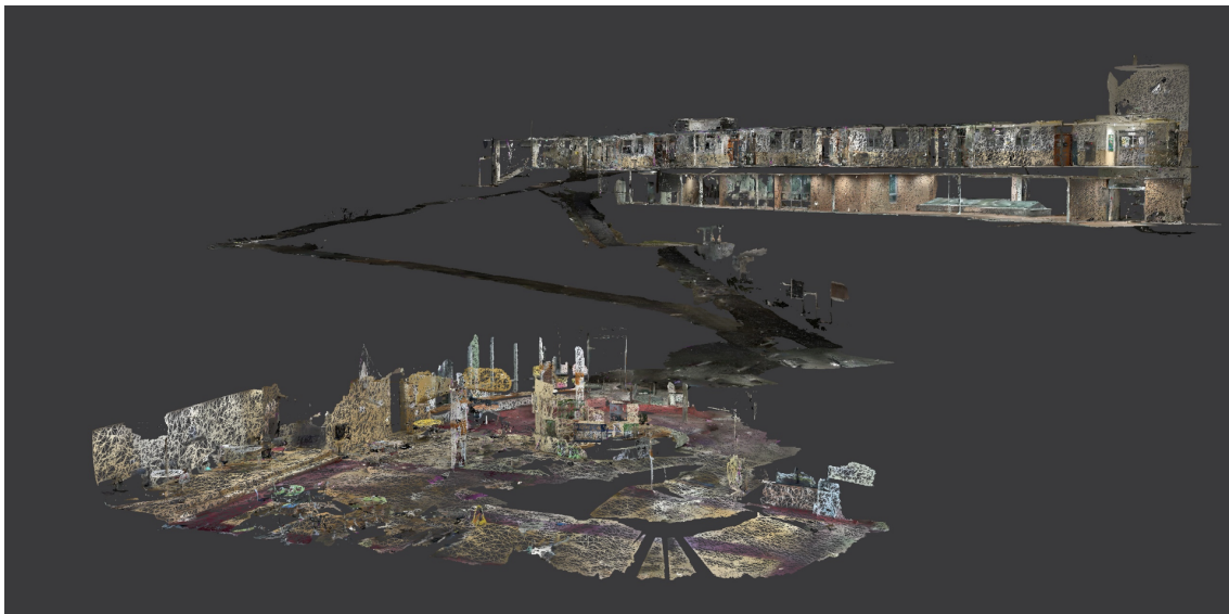
[fig 4-5] Lidar 3D Scanning Data with Texture(Image Data) (Veritas hall 3F, 4F and Lux hall 1F)
